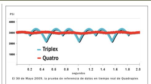
Figure 3C. Live recording of the quadraplex mud pump output pressure curve
