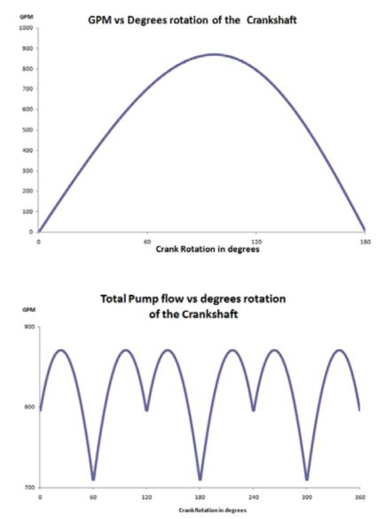
However, the maximum flow in the cylinder at the peak speed of 380 fpm is 871 gpm, more than three times the cylinder average flow rate.
